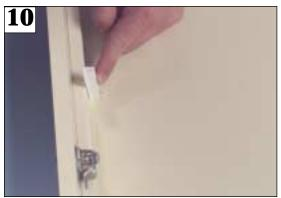
10. Using another holder, peel away the adhesive backing and press the holder to the mark on the front of the drawer.
