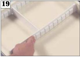
19. Attach another grooved strip on the right side of the front to back divider strip.
