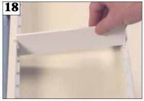
18. Mark, score, and break another divider to fit between the grooves. See steps 12-16. Slide the divider strip between the grooves on the grooved strips.
