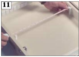
11. Measure the distance from the center of the back holder to the center of the front holder.
