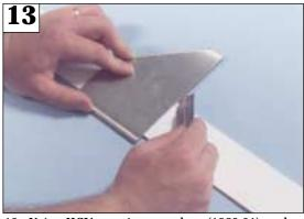
13. Using HCL's cutting template (1859-01) and retractable knife (1860-01) score the divider strip 3 to 4 times on the mark. (a straight edge and utility knife will work)
