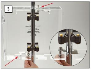
**Step 3.** Press and twist the safety latches located at the top and bottom of the box to the locked position.
