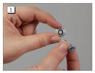
**Step 1.** Take both bolts and place a washer on the end. Make sure the shiny side of the washer is facing the bolt.
