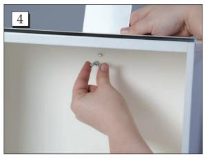
**Step 4.** Now fasten the bolt in place from the inside of the box with a wing nut. Repeat step 3 and 4 on the bottom hole.
