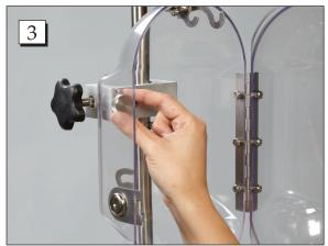
**Step 3.** Tighten the locking wheel on the inside of the pod.
