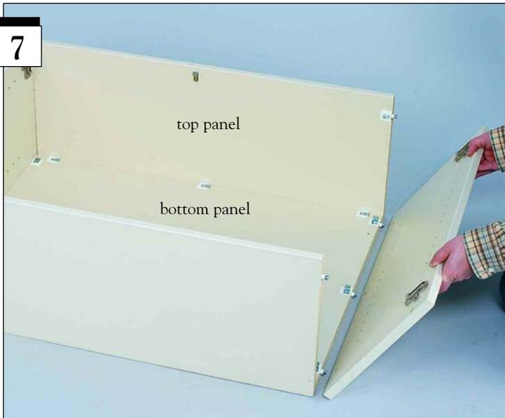
Attach the right side by aligning the pre-drilled holes with the connection fittings in the back, top and bottom panels. Push the panels together and press the fitting toggles down to secure.
