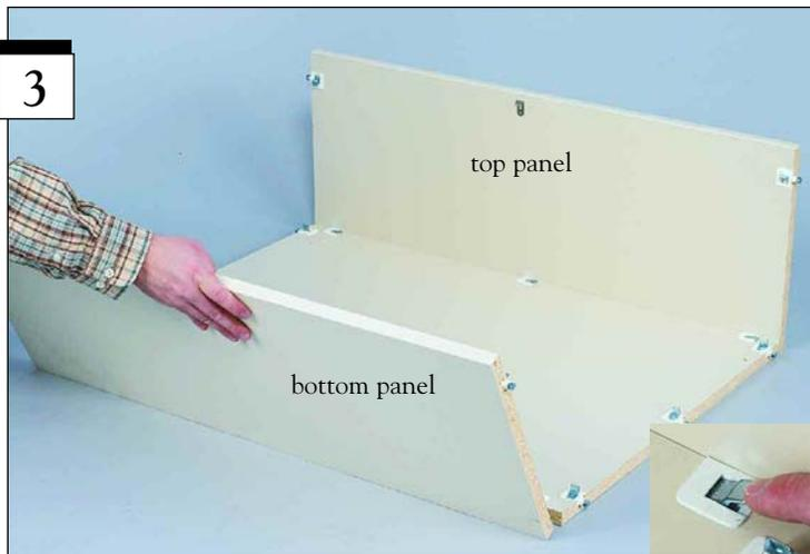
Attach the bottom panel by aligning the pre-drilled holes with the connection fittings in the back panel. Push the two panels together. Once together, press the fitting toggles down to secure.
