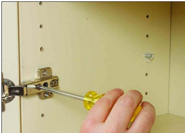
**The left adjustment screw provides depth adjustment:**
