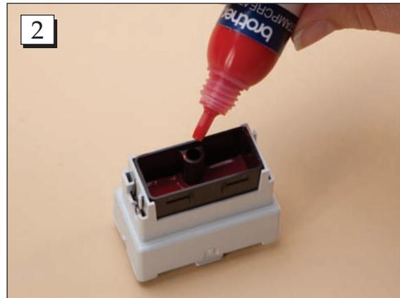
**Step 2.** Put five drops of ink into each of the refill ports as shown.
