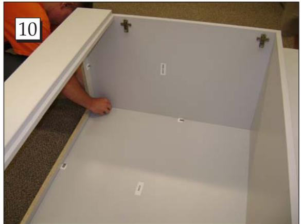
**Step 10.** Push the panels together and press the fitting toggles down to secure.
