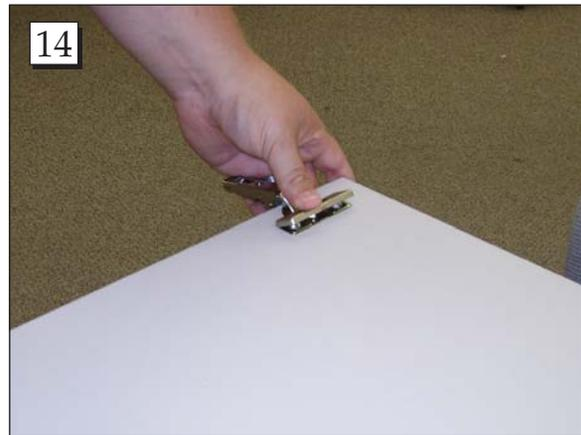
**Step 14.** Once hinges are in place and flush against doors, press down on the screw cover plates to secure hinges to doors.
