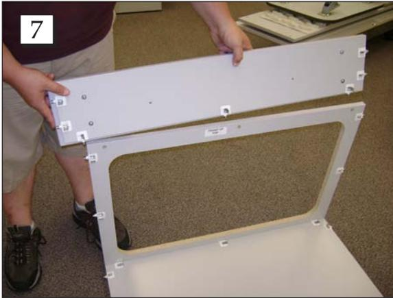
**Step 7.** Attach the front panel to the inside of the top panel.
