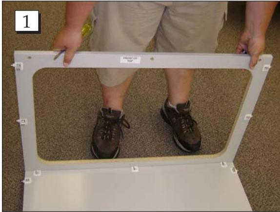
**Step 1.** Lay the back panel flat on the floor. Bring the top panel into position.
