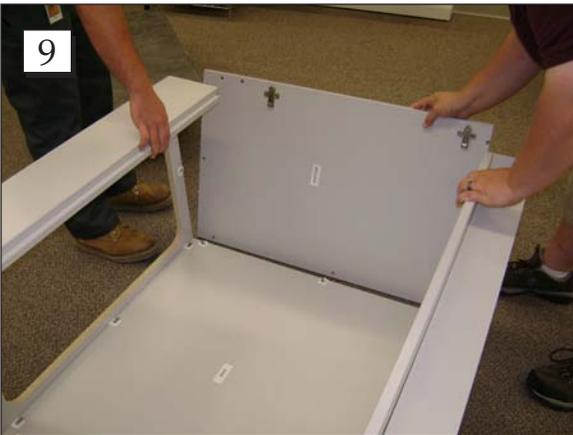
**Step 9.** Attach the right side by aligning the pre-drilled holes with the connection fittings in the back, bottom and top panels.
