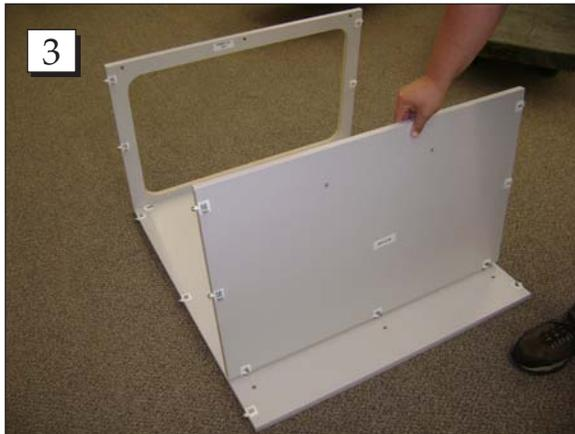
**Step 3.** Locate the bottom panel and position at the bottom of the back panel. Attach the bottom panel by inserting the connection fittings in the bottom panel into the pre-drilled holes in the back panel. Push the two panels together.
