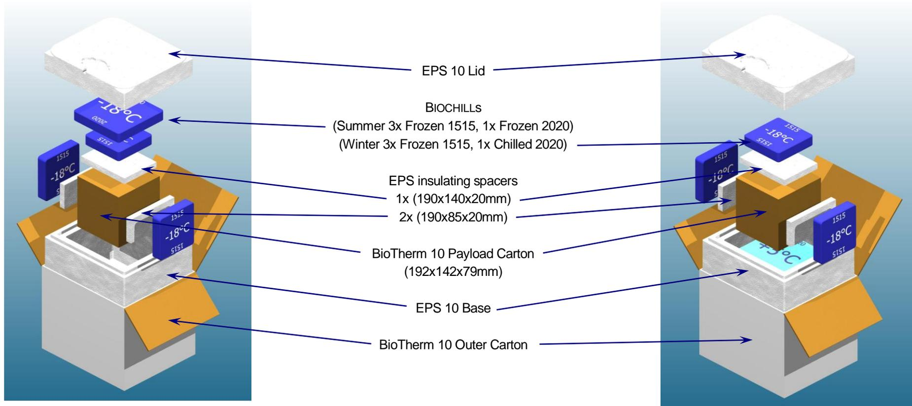
Chilled BIOCHILLS should be conditioned at +5°C for a minimum of 24 hours before use. Frozen BIOCHILLS should be conditioned at -18°C for a minimum of 24 hours and then for approximately 20 minutes at factory ambient +20°C (± 5) before system assembly.
