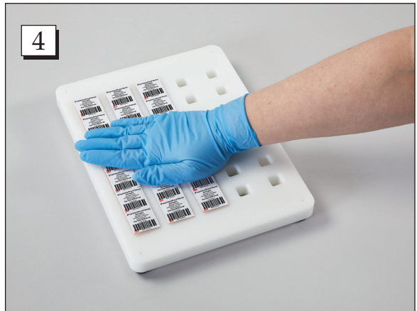
Step 4. Press the labels onto the blisters.
