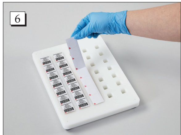
Step 6. Remove the blisters from the sealing tray.
