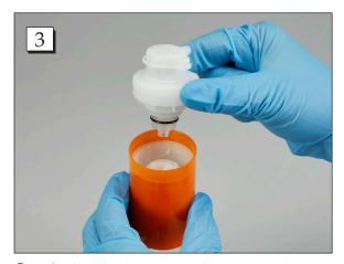
**Step 3.** Place the actuator into the opening of the pouch.
