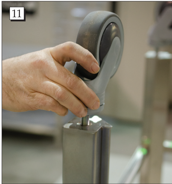
Step 11. Tighten the 4 casters into place.
