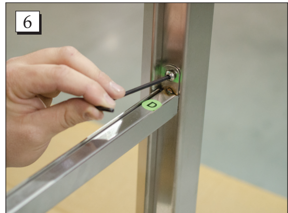
Step 6. Secure each side of the short support bar with a button head screw. Tighten the button head screws with the provided Allen wrench.
